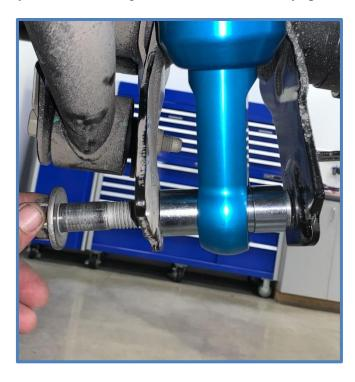
5. <u>Mounting Reservoirs</u> – First attach the reservoir clamps to the reservoir brackets as shown below. Install the 1/4 X 1/2" BHCS (CB2420) with red locktite and tighten using a 5/32 Hex Key.
