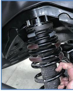
3. <u>Install King Shocks</u> – Be aware the shocks are side specific, make sure you are installing shocks on the proper side. See photos for proper orientation. Place the shock into the upper mount and install the 3/8 Heavy Duty washers (CW1701) and 3/8 nuts (CN2711) on upper mounting studs and tighten to 35 ft/lbs.
