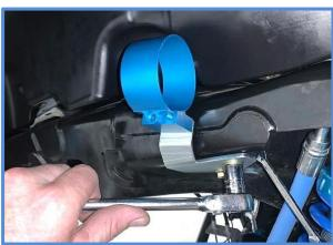
7. Slide the reservoir into the reservoir clamp. Install the 1/4 X 1" bolts (CB1501) in the reservoir clamp and tighten using a 3/16 Allen wrench.
