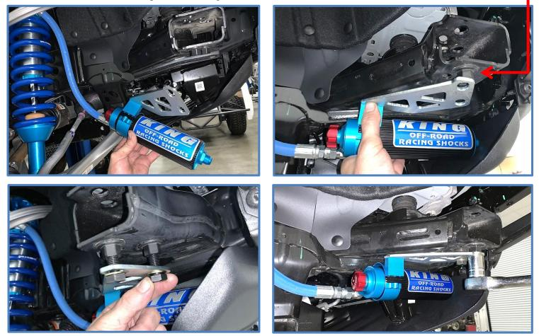
19. Install the 1/4 X 1" bolts (CB1501) in the reservoir clamp and tighten using a 3/16 Hex Key.
