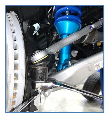
12. Reconnect the upper control arm and tighten to factory specs.
