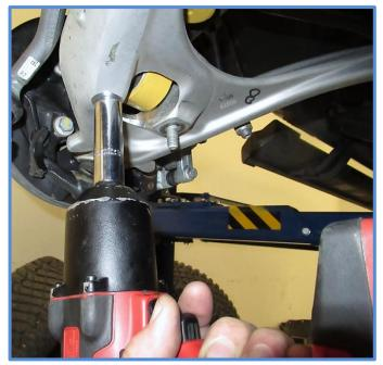
3. Remove the upper mounting nuts using a 15mm wrench or socket.
