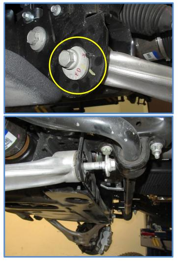
Place the lower control arm back into the lower mount and install the cam bolts to the same position prior to removal. The vehicle will need to be aligned properly after the install but keeping the factory settings will get you to the alignment shop. Tighten lower control arm bolts to factory specs after the vehicle is sitting back on the ground. Removing right shock should not require removing lower control arm bolts. Remove right shock and move to next step...
