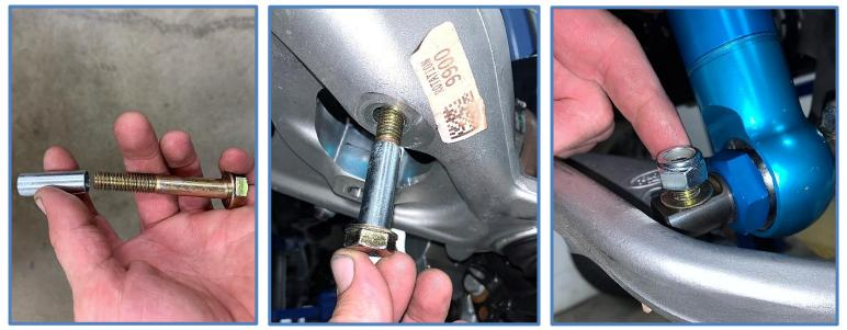
11. Reconnect tie rod and tighten to factory specs.
