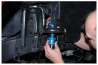
12. Once the cutting and trimming is complete you can mount the bumpstop. The bumpstop position locates on the upper ring. With the bumpstop in the mount, turn the upper collar on the threads until one thread is showing above the collar. This properly positions the bumpstop in the mount. Tighten the lower collar by hand.
