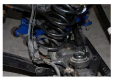
15. Push the coil spring up into the top mount making sure that the coil is indexed to the lower mount as shown.
