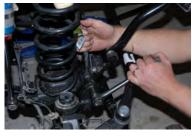
3. Remove the swaybar links from both sides and unbolt the shocks.
