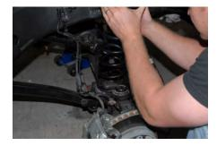
16. While pushing down on the front axle move the bottom of the spring onto the lower mount. Make sure the end of the bottom coil sits in the relief on the lower mount.
