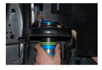
11. Time to do a trial fit. Push the bumpstop up into the mount and thread the top collar on. The bumpstop locates on the top of the mount. Making sure that the top collar is flush with the top of the mount inspect the bottom edge for any high or low spots that need to be trimmed. Mark those areas and carefully trim them until the lower bumpstop collar sits flush with your cut edge.
