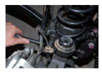
1. Remove the bolt holding the brake lines as shown.
