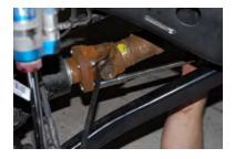
4. Brace the driveshaft so it does not rotate and remove the 4 bolts holding it to the flange.
