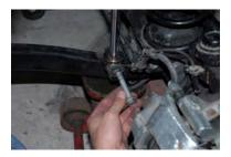
21. Insert the shaft end into the lower mount and replace the bolt, washer and nut and tighten. Tighten the top nut until the bushings begin to compress,
