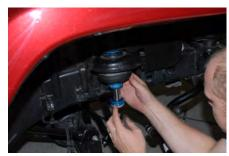
14. Now you can put the suspension back together. First slide the rubber coil spring isolator over the end of the bumpstop.
