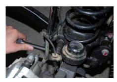
18. Replace the bolt through mount and thread into the captured nut and tighten.
