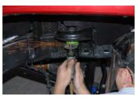
9. Before cutting remove the shock. You can use a sawzall or cutting wheel to make the cut. Make sure you wear a face sheild and cut as straight and level as posible.
