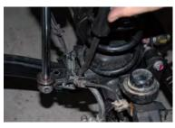
2. Gently pry the bracket out on the end closest to the bolt.
