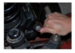
19. After performing the same steps on the opposite side, bolt up the swaybar ends and the driveshaft.
