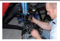
6. Push down on the axle and remove the springs starting on the passenger side.
