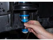
13. Using a puch gently tap the lower collar until it is tight. Apply locking compound on the supplied set-screws and tighten them into the threaded holes on the top and bottom collars.
