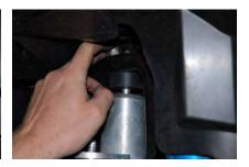
20. The lower rubber bushing and sleeve should be on the mounting pin as shown. Place the top rubber bushing, blue anodized plate and flat washer over the whole in the top mount and push the shock up into the mount. Thread the nut on the protruding pin.
