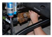
5. Pull the driveshaft back and let it hang down. You need to do this so the front end can droop fully.
