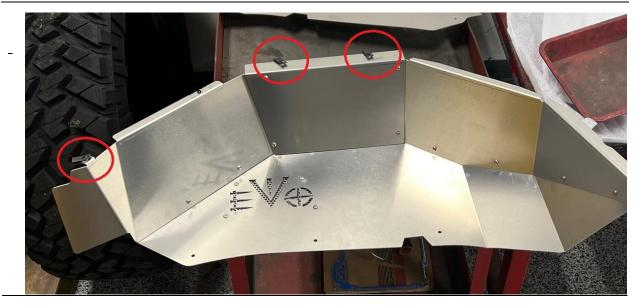
Before installing to vehicle, rotate clips as shown and use supplied ¼" screw to center clips in holes making sure bolt will thread.
