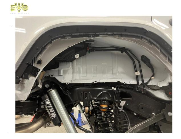
Additionally, clip/remove the 1 clip as shown.
