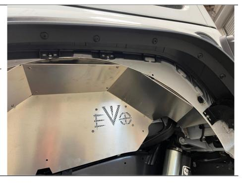
Center Mark forward mounting how and drill with 9/32 drill.
