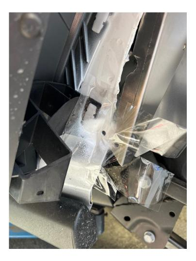
Install supplied  $\frac{1}{2}$  screw with washer and nut on the forward drilled hole.
