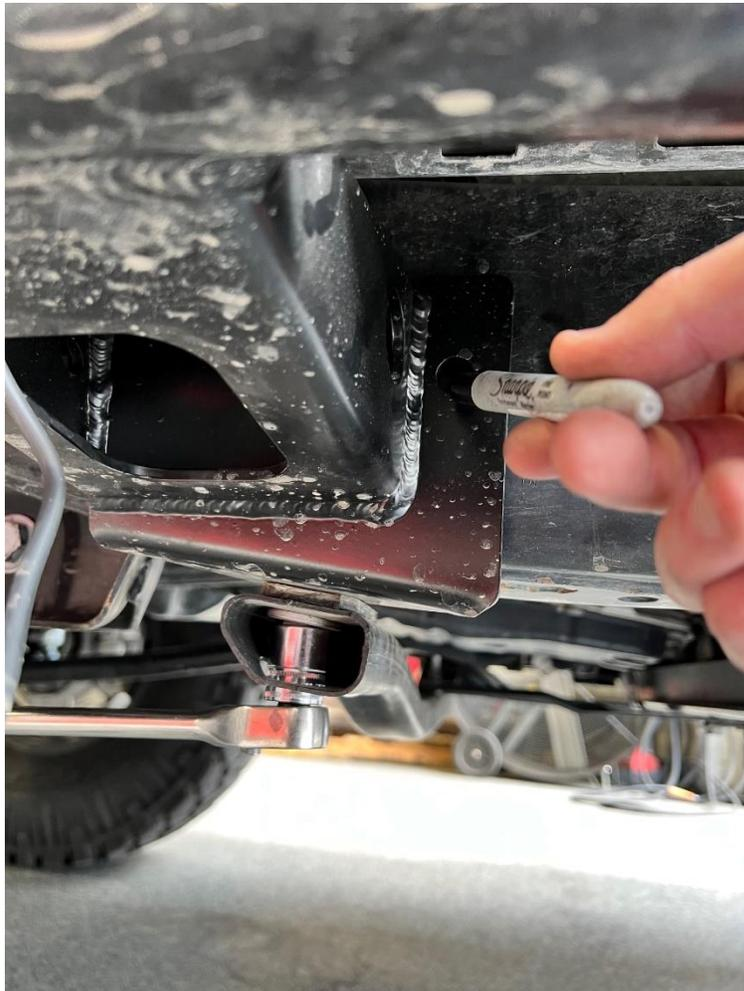
Remove the factory hardware installed on the underside of the frame and the 2 installed nut plate, use vice grip/hold tab on nut plates before bolt removal to prevent tab from falling into frame. Remove slider from vehicle.
