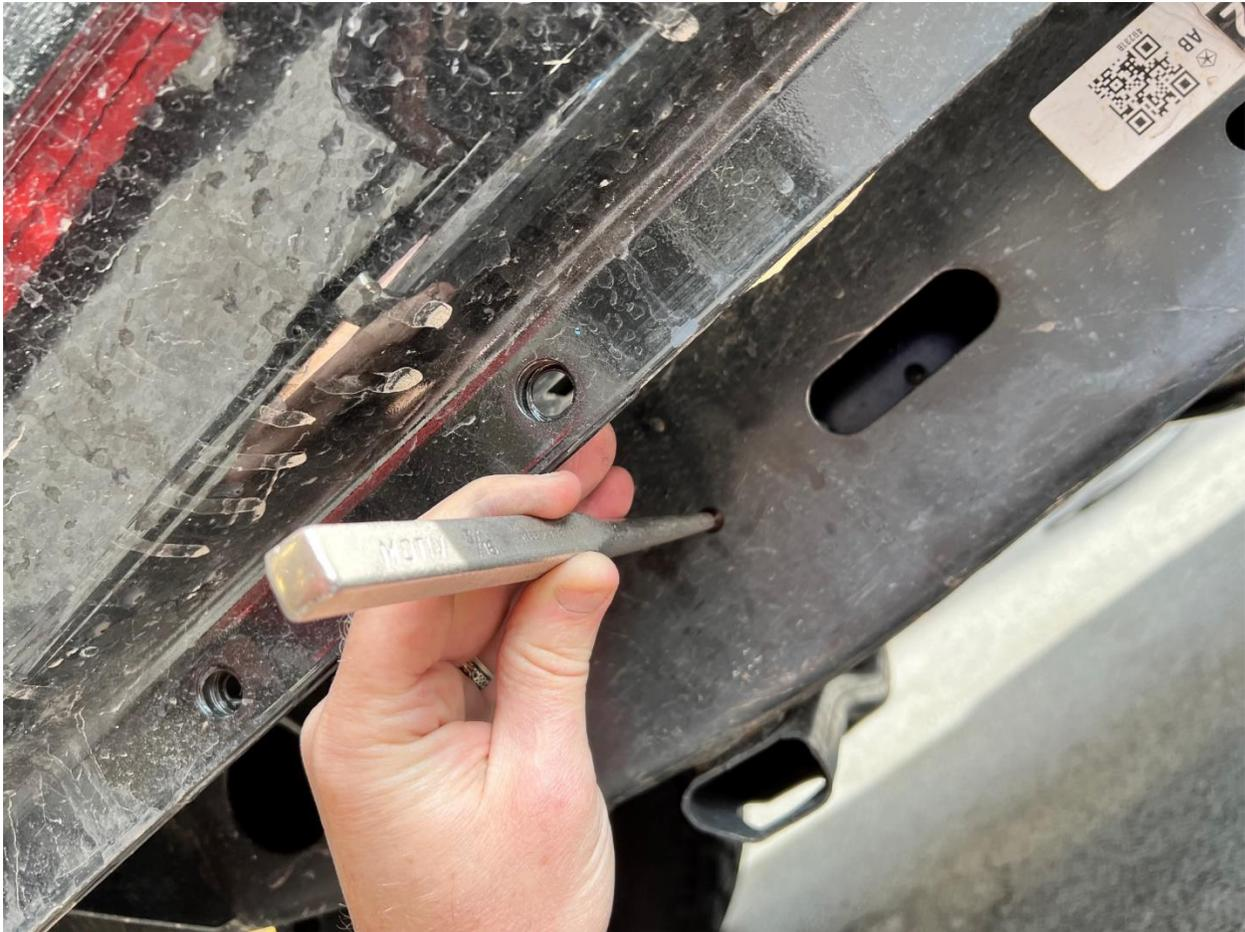
The final drill size of all drilled holes 15/32"-1/2" drill bit. Start with smaller drill on all holes and then step drill size up to final size. Drill all 4 marked/center punched holes.
