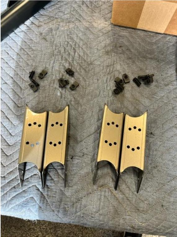
End Plate Assembly: With a firm push, press on nut clips to Slider End Caps over the 4 holes of each part. Barrell section of nut clip should be on the inside of the part all 4 places. Center clip thread over holes.
