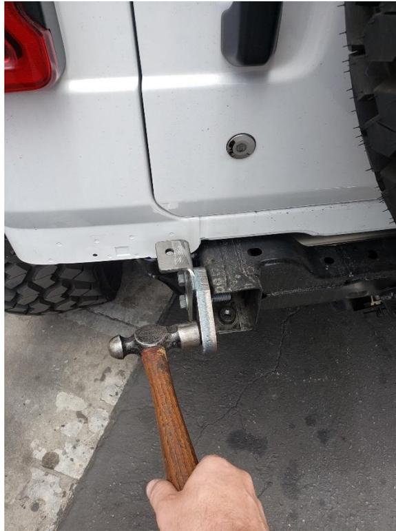
Be cautious of sensor wiring. Do not pinch wires when installing bumper.
