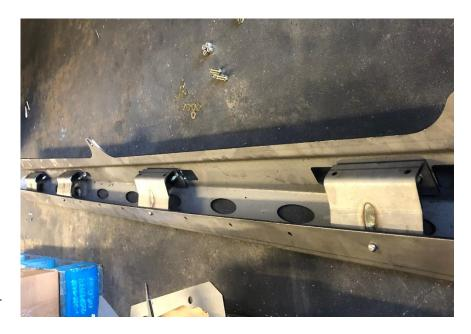
3. Using the supplied 3/8" hardware, loosely install all 8 bolts from bottom up at all 4 inner seam mount locations (2 each mount). It is best to tighten these to the point just before getting tight (loose but almost tight). This will save time later during final install while tightening all bolts on the vehicle.
