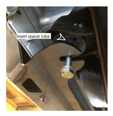
Using the factory holes in body pinch seam install supplied 5/16" bolts and washers through body and into inner seam mounts.
