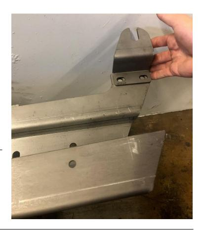
5. Install all button head bolts into bomber bolt hole locations (see picture for reference.
