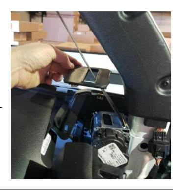
19. With a sharp and firm pull, pull main panel away from side of vehicle.
