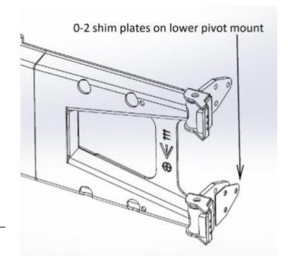
26. Swing tire carrier towards tailgate and route wire for camera and brake light (if applicable as shown through carrier holes) out of camera tube.
