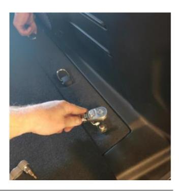
17. Remove single screw in rear trunk panel on side of vehicle just rearward of rear passenger door jam.
