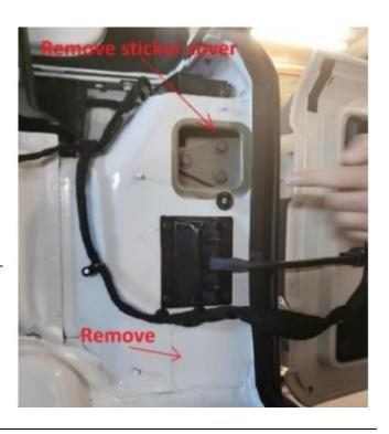
21. With tailgate closed and rear window open, using a Torx Bit (T55) remove the 2 bolts holding the hinges to tailgate, both top and bottom. From here out it is recommended to not open the tailgate until complete.
