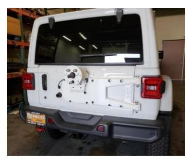
34. Loosely install the supplied 7/16 bolts, washer nuts into the 3 slotted holes.
