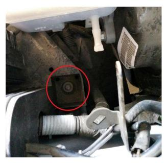
12. With the upper tab secured, tighten the nut on the rear tab from step 8 using a 10mm socket and extension (Same as step 7).
