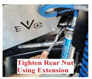
8. On the Driver side, fit the Mini EVO Liner's rear bolt tab to the bolt stud and thread on a nut as before, however, you will need to be sure the bolt tab fits underneath the brake line, as shown below.
