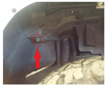
Remove the panel clips using a panel clip tool or similar tool. There are a total of
