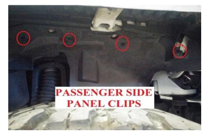
4. On the Passenger side, fit the Mini EVO Liner's rear bolt tab to the bolt stud holding the electrical connectors in place, shown below. Thread the supplied nut on, do not tighten it at this time.
