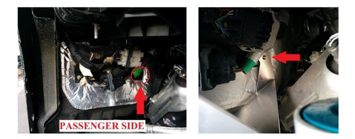
5. With the rear bolt tab in place, fit the Mini EVO Liner's front bolt tab to the bolt in the upper part of the wheel well, shown below.
