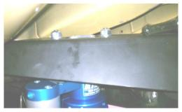
Install the supplied M10 nuts and washers to the shock bolts above the EVO strengthening plate.
