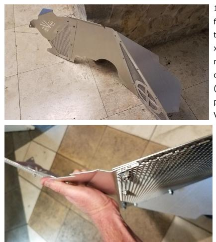
1. Assemble Inner fender parts on table prior to install. Use supplied #10 x 1/2" bolts and nylock nuts. Each inner fender is comprised of 3 main pieces (front middle rear) and 2 perforated vents (DTD Version is one piece with 2 vents, for this use supplied hardware to directly mount vents to back side of each liner). During assembly of liner, front and rear piece must be mounted on outside of inner piece. At this connection of parts, the
