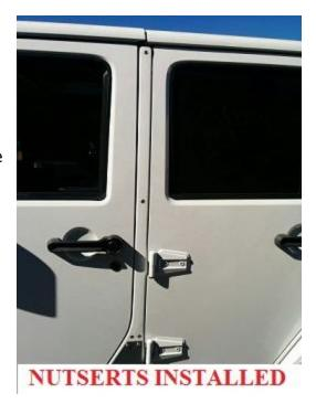
Note: The B-Pillar Rockskins come with 2 sets of hardware to match armor on your vehicle. If your vehicle has flat head hardware (EVO MFG Rockskins) install The B-Pillar Rockskins with countersunk holes facing out to fit the flat head hardware. If your vehicle has button head hardware (EVO MFG Boatside Bombers) install the B-Pillar Rockskins with the counter sunk holes against the body (flat side out).
