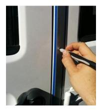
3. Only if you are satisfied with the position of the B Pillar Rockskins, center punch and then pilot drill all the holes into the body sheet metal. You only want to drill through the surface layer of sheet metal, and no deeper.
