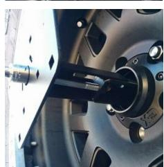
4. Use a 9/16 socket with extension to tighten the Mounting Plate until it is flush with the tire.
