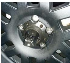
Slide the Mounting Plate over the Stud Plate and thread the 4" long bolt through and into the nut in the stud plate
