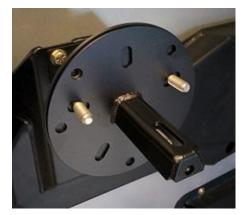
2. Install the spare tire, sandwiching the stud plate between the tire and tire carrier. Tighten the lug nuts to the studs.
