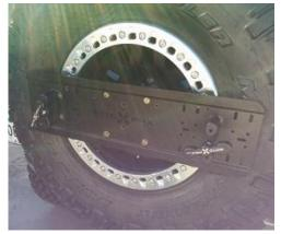
6. The mounting hardware or gas can needs to be pulled tight against the tire to apply tension and keep the gas can from rattling. You will need to use a 9/16 wrench (a ratchetting wrench works well for this) to tighten the bolt until it does. This bolt can be accessed from the underside without removing the RotoPax hardware.
