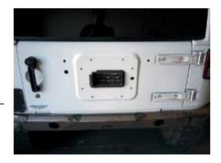
6. With the tailgate closed and your vehicle on level ground, remove the factory hinges by removing the 4 bolts on the tailgate (13 mm wrench) and the 6 bolts on the body (Torx T50). Set bolts aside to reuse later.
