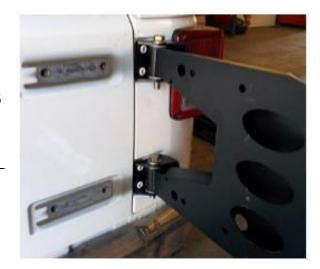
9. Using the 4 bolts that mounted the factory hinges to the tailgate in step 5, slide them into the 4 holes from the outside as shown. On the top, hang 1 of the supplied oval spacers and on the bottom, hang 2 spacers from the inserted bolts as shown.
