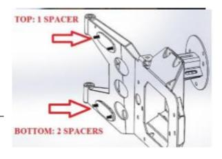
10. Slowly swing the Tailgate Tire Carrier closed being sure the bolts and spacers stay in place. As the Tire carrier comes flush with the tailgate, make sure the 4 bolts line up with the 4 holes in the tailgate. Use a 13mm socket with extension to thread the right side bolts first, then the left. Do not tighten them at this time.
