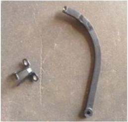
22. Reinstall the door catch with the new bracket. Start by loosely bolting the door catch back with the new bracket and supplied washers as shown. While holding the catch in place, gently close the door until it is reinserted into the vehicle body. Once the catch is back in place, open the tailgate and slide the bracket all the way toward the vehicle and tighten the screws as shown.
