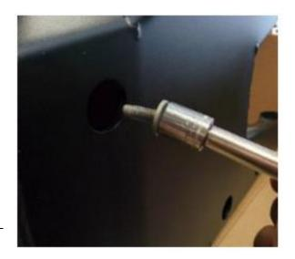
Note: If you don't have an extra-long T50 bit, this install can still be done, but it may require 2 people. After completing step 12, start by opening the tailgate and applying upward pressure on the tire carrier and tailgate. Tighten the bolts on the inside of the hinges (Pictured in step 14). You then need to check and verify that the tailgate closes and latches properly. If it does not, loosen the bolts, adjust and retighten. It may take several tries.
