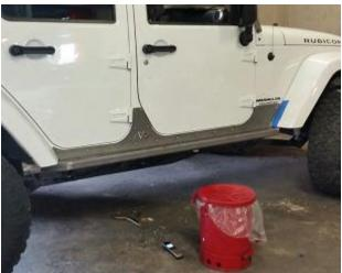
17. With raw parts installed and fitting correctly, remove the Boatside Bombers and have them powder coated, or otherwise treated to prevent rust. Repeat steps 10 and 11 to reinstall.
