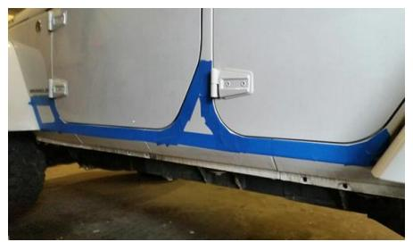
3. Using an 18mm wrench, remove the bolts from the 3 body mounts on each side. Mark each bolt with the mount location that each came from.
