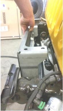
10. Using the included winch mount spacers and winch mount nut plates install the EVO winch mount plate to the factory frame rails. The winch plate spacer should be positioned in-between the EVO winch plate and factory frame rail. Depending on customer clearance of factory vacuum pump bracket, a spacer may or not be needed on the driver side. The EVO winch mount nut plate should be installed in the pocket along the factory frame rail. Do not tighten at this time
