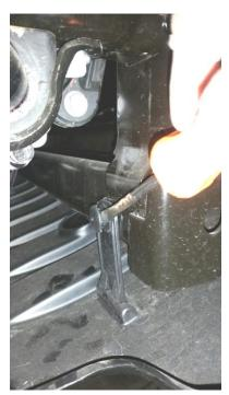
**3.** Remove factory bumper with an 18mm socket, there are 8 nuts total that will need to be removed.
