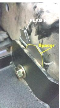
**11.** Using a 17/32" Drill bit drill out the driver side upper outer side frame horn mount hole.
