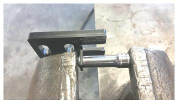
vice, align bolt straight with hole. Press/vice bolt into hole making sure bolt stays as straight as possible while inserting. Repeat steps for the other mud flap frame mount.
