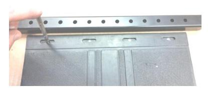
7. Holding one of your mud flaps up to the EVO mud flap tube mark the holes on the EVO mud flap tube that best suit your tire coverage needs.
