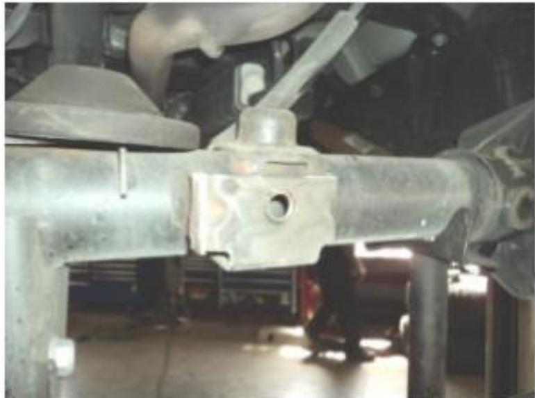
27. Install rear trackbar bracket as shown with supplied 9/16 bolt and u-bolts.
