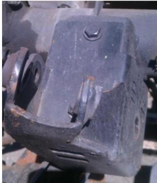
22. Reinsert lower control arm into the axle mounting brackets
