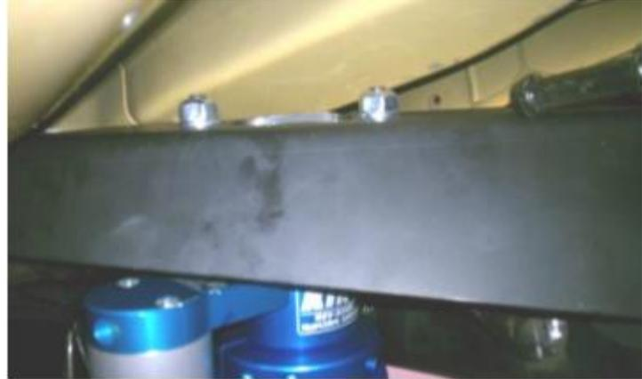
31. Install the supplied M10 nuts and washers to the shock bolts above the EVO strengthening plate.
