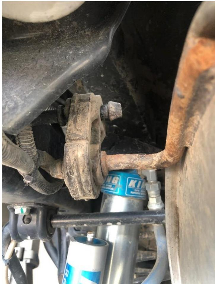
12. On passenger side rear exhaust hanger at frame. Bend hanger upwards about  $\frac{3}{4}$ " with pry bar.
