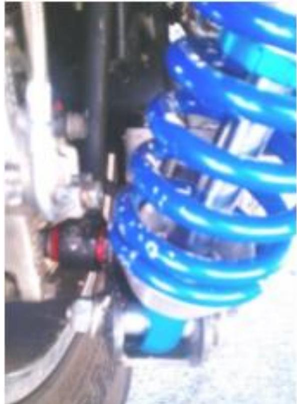
35. Remove Factory Swaybar from frame. Two bolts each side.
