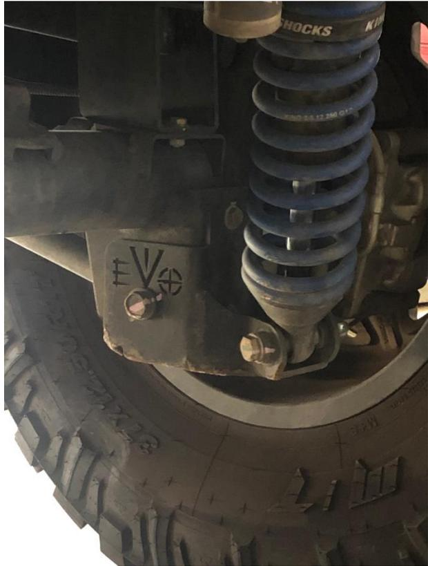
24. Remove rear trackbar bolt at axle, leave trackbar bolt at frame installed
