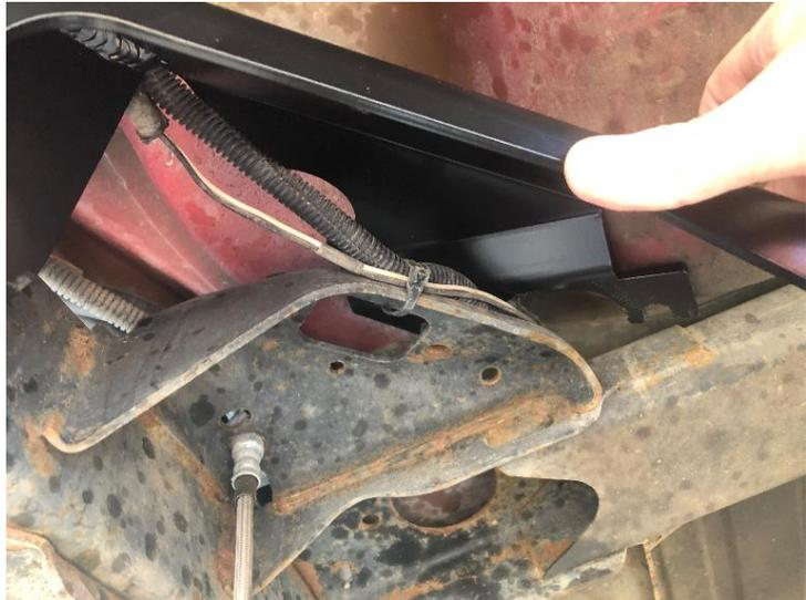
15. After strengthening bracket is inserted. Lower Jack, tighten all body mount bolts.
