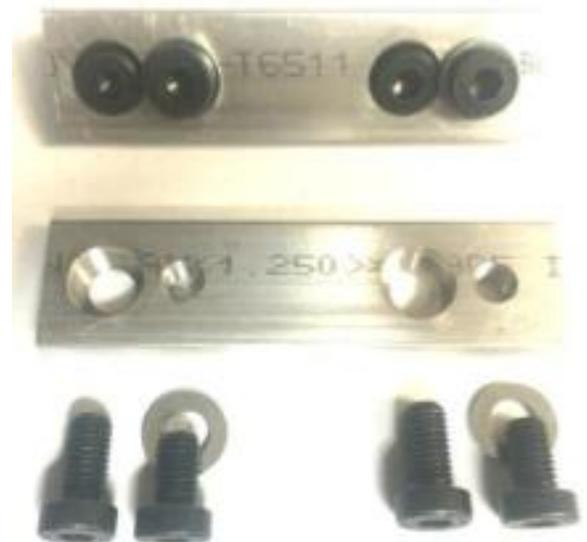
37. Re-Install OE Swaybar to EVO MFG Swaybar Relocation Spacers using 2x 16MM Black Hex Bolts and a washer on each bolt. Repeat on opposite side of vehicle.
