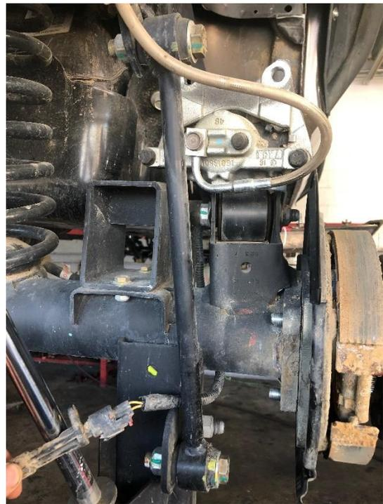
6. Remove both driver and passenger side shocks.
