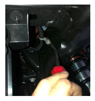
17. Lower jack under axle giving room to remove rear springs. Be sure that springs can be easily removed, forcing the springs out when under any load is not recommended.
