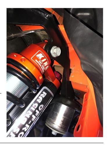
24. Tighten supplied 3/8" (rearmost) bolt and nut. Use table at bottom of instruction for proper torque specs.
