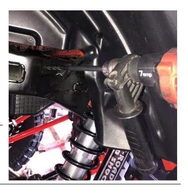
19. Using a 16mm retracting wrench remove factory bolt, retain for later use.
