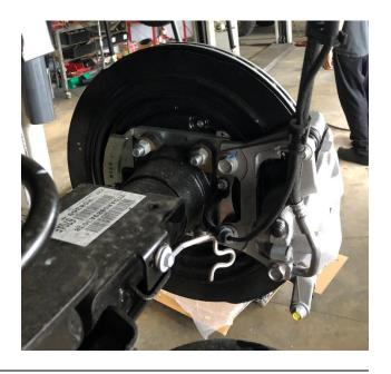
35. Moving swiftly/carefully separate the hard line from the bracket/hose on frame by holding hardline with a 12mm wrench and unscrewing the rubber hose with a 16mm wrench.
