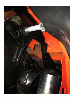
21. Loosely reinstall the body mount bolt, using a 16mm socket, through the EVO MFG reinforcement bracket and into the body mount bracket.
