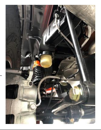
Note: Carefully move line. Do not crimp/pinch line. Always check for leaking fluids and that brakes work correctly. Bleeding brakes is extremely important to be done properly. Follow factory specifications in doing so. Consultation/should be performed by a trained professional mechanic.
