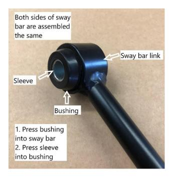
26. Install sway bars using factory hardware. Make sure axle side sway bar links are attached on inside of factory sway bar.
