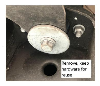
24. Fit bracket to frame on left and right of vehicle using the single factory bolt on lower side of frame. This bolt is the bracket locator on both left and right sides.
