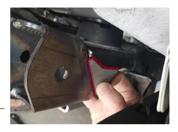
27. On rear axle, cleanly cut and grind smooth to axle tube the entire driver and passenger side rear lower control/shock mounts.
