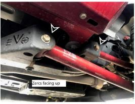
Install supplied 3/8-24 bolts and washer nuts on all arms at pinch locations
