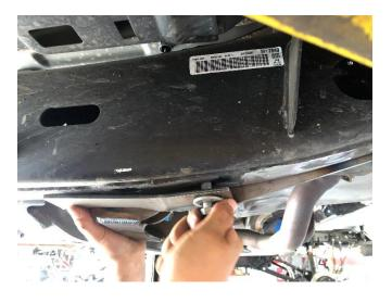
19. EVO-3010 3.6L GAS Models Only. On driver side front only, lower arm mounting hole will need to be drilled through frame. Mark center using bracket as template and drill through both sides frame using a drill similar in size to your hole saw centering drill bit (~1/4" drill). Bracket may need to be removed to drill. Be careful to keep drill as square and centered while drilling outer frame material. EVO-3010D: DIESEL/392 KIT Will OMIT THIS STEP.
