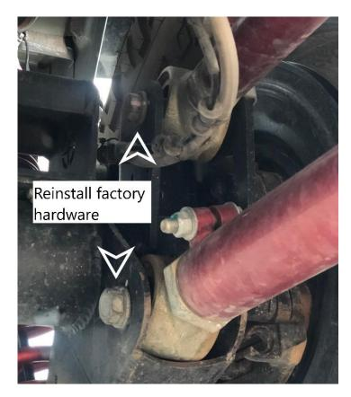
33. Rear Lower will used supplied 4" x 9/16" bolt, washers and small flag nut on both driver and passenger side frame. \*Rear Upper will used supplied 3.5" x 9/16" bolt, washer and small flag nut on both driver and passenger side frame.
