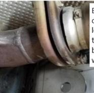
Bolt installed, tap center of inside lower bracket hole then drill through both sides of frame with ~1/4" bit
