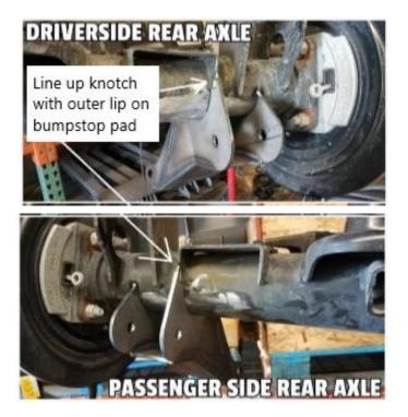
Once positioned, tack in place. Verify correct location of left and right and weld all connections to axle. Both sides.
