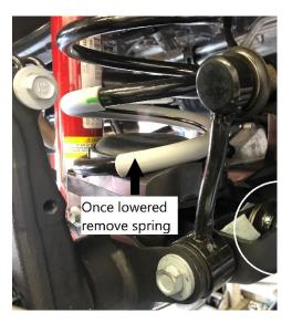
Remove upper control arms from frame and axle and set aside. Axle will be loose at this time use caution and appropriate support.
