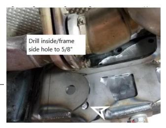
21. EVO-3010 3.6L GAS Models Only. On outside of frame we need to make a relief hole to install nut and washer inside frame to newer lower control arm bolt. Using at 1" or larger hole saw and the previously drilled pilot hole make hole in OUTSIDE of frame ONLY.
