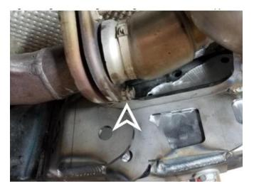
18. Once all control arm mounts are clearance clean to frame. Starting in the front install front driver long arm bracket to frame using the single bolt hole on the underside of the frame, where exhaust bar was once bolted, using original factory bolt. This will locate this bracket in the proper location. Slight clearance of edge/lip on exhaust collector may be required. Do so as needed.
