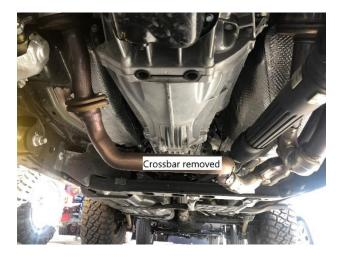
16. Using tools at your deposal, grinders, cut off wheels, torch, plasma cutter etc. Clearance all control arm mounts, front upper, lower and rear upper and lower clean to frame rails.
