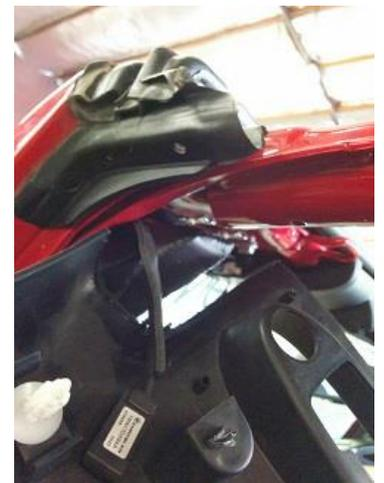
23. Slide the Driver side connector plate (pictured with bolt flap facing up) between the top of the A-Pillar support and the windshield frame making sure the holes on both align with the threaded hole in the top of the windshield frame. The connector plate should be sandwiched between the windshield frame and EVO A-Pillar Support.
