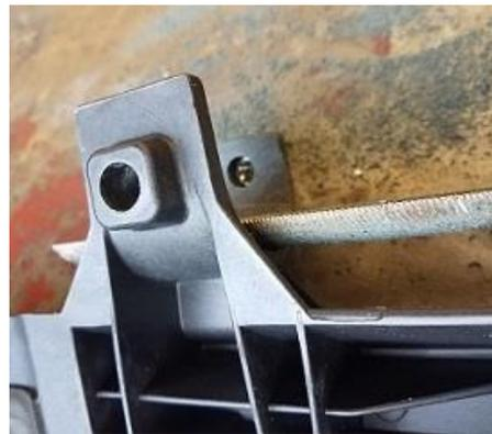
46. Install the door surrounds and verify the fit. If necessary, sand/file again (this may require multiple iterations to achieve an acceptably fit). Note: depending on the holes drilled through the tubes, the C-mount may need to be cleared around the bolts/washer.
