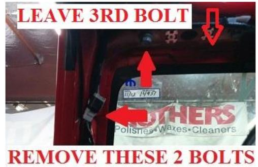
12. If equipped, remove panel clips holding the wiring harness to the windshield frame. Wiring should be free, as shown.
