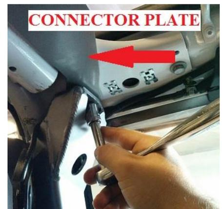
25. Using a 13mm socket, thread one of the bolts removed in Step 11 through the A-pillar support and into the side of the windshield frame. Do not fully tighten at this time
