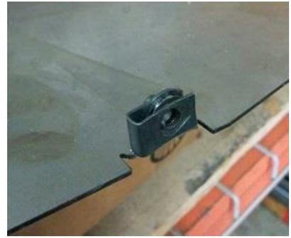
34. With the clip nuts installed, put the closeout in place and use a 1/8 Allen wrench to thread the black button head cap screws through the Center Bar and into the clip nuts.
