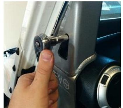
30. Thread 2 of the supplied black button head screws through the 2 small holes near the bottom of the A-Pillar Support and into the clip nuts installed in Step 18.
