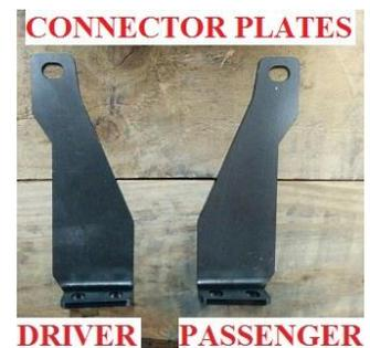
24. With the wiring in place, use a 13mm socket to thread the supplied M8 bolt through the A-Pillar support and connector plate and into the top of the windshield frame. Be sure to tighten this enough to pull the A-Pillar Support all the way up to the top of the windshield frame, but do not fully tighten at this time. The A-pillar should be lifted to the windshield frame but still relatively loose.
