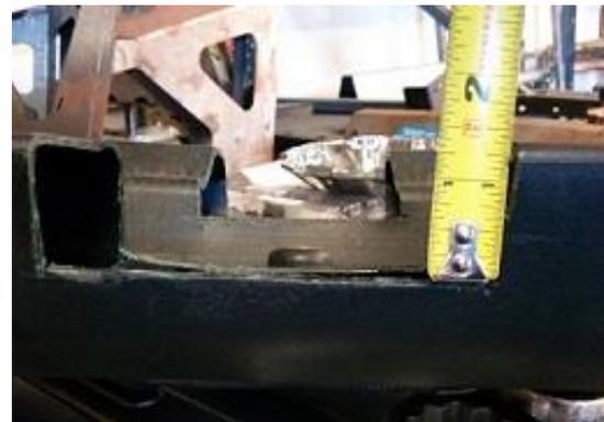
38. Connect your marks and carefully make your cuts. Be very careful not to cut the wiring in the rear of the bar. Depending on the year, it may be wrapped in foam (pictured) or may be exposed. Make shallow cuts to avoid damaging this wiring.
