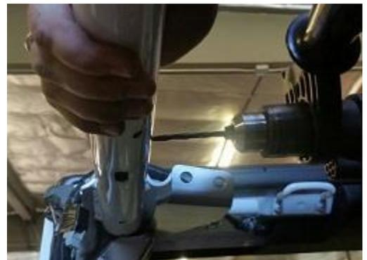
29. Slide the Upper Cross Bar back into place and reinstall the Center Bar. 1<sup>st</sup> thread 2 of the supplied 3" bolts, washers and locknuts through the holes drilled and the outer bolt plate on the crossbar. With these threaded, thread the supplied
