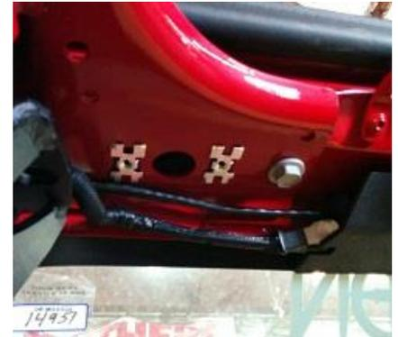
22. If equipped with a microphone, you will need to plug this back into the wiring harness before bolting the A-Pillar support back into place. Make sure this wire comes out on the outside as shown. The plastic fascia from Step 20 will need to be trimmed before the microphone is plugged in.
