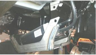
Loosely secure the front of the EVO Evap Main Skid with the two factory front evap bolts, leaving a few threads showing.
