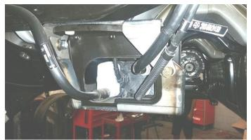
7. Tightly secure the two factory front evap bolts and the one factory rear evap bolt.
