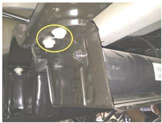
2. Loosen and remove the rear factory evap skid bolt completely.
