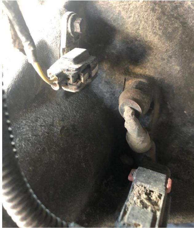
5. Support axle with jacks and remove rear sway bar end links from vehicle. (upper stud end on sway bar link has hex key on end of the stud to prevent rotation while removing nut).
