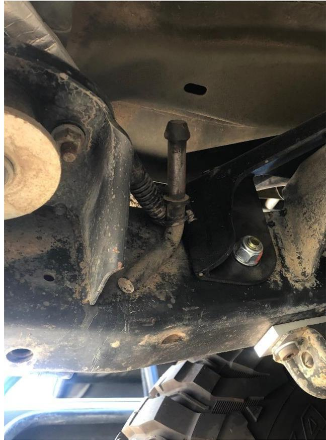
13. Using a jack, carefully apply pressure to rear tub lifting rear of body from frame. There needs to be about a  $\frac{1}{2}$ " gap between body and frame.
