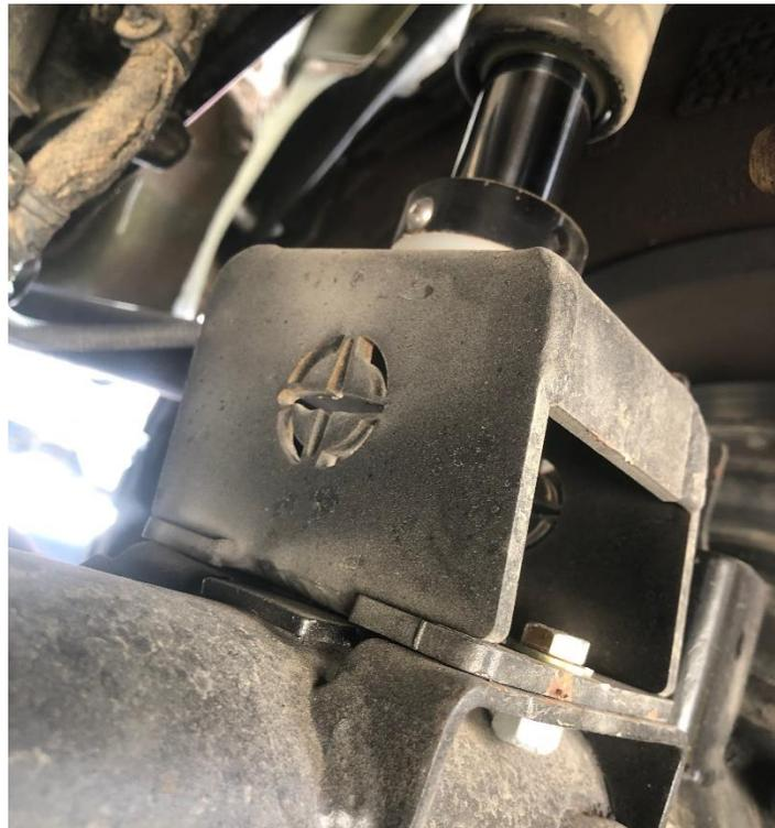
30. Using supplied socket head bolts, thread two mounting bolts into stock threaded frame bolts. This needs to be done in iterations. Walk the bracket up by threading one bolt a few turns then the other and continue until fully seated. Bolts need to go through 2 holes in the EVO upper strengthening brackets.
