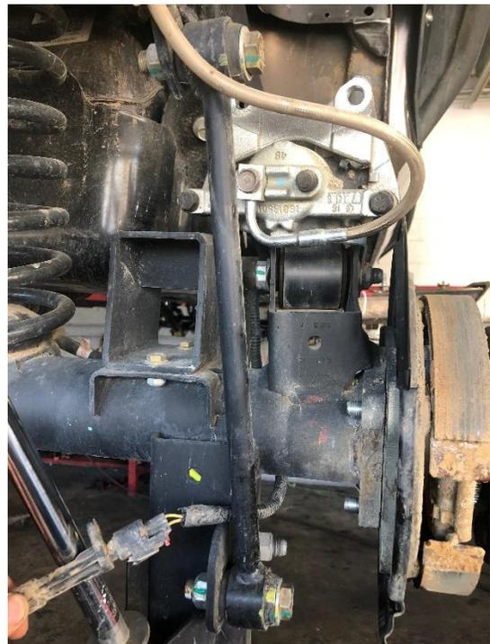
6. Remove both driver and passenger side shocks.
