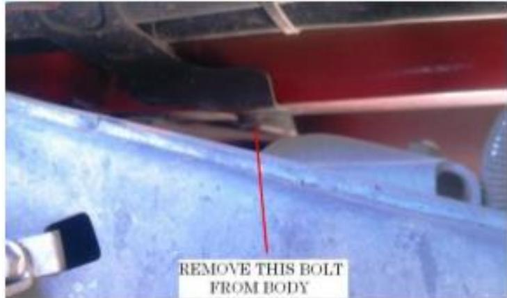
11. Remove muffler from vehicle. Loosen clamp just in front of axle on the exhaust. Spray lubricant on rubber hangers, pry hangers from frame.
