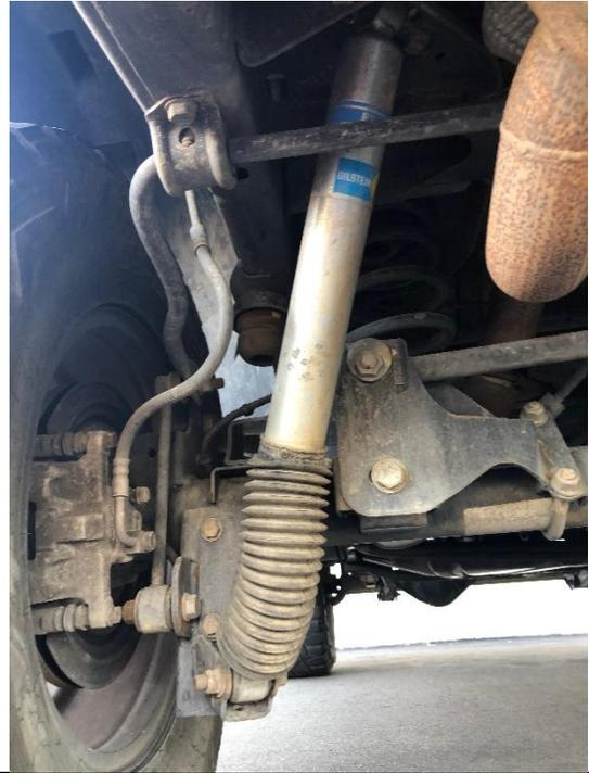
7. Lower axle until springs can be removed. Remove rear springs and upper/lower coil isolators.
