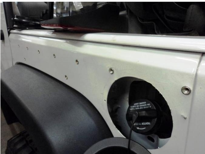
9. Install nutserts into drilled holes. Fully thread the long 1/4" bolt with nut into the nutsert as seen in photo. With wrenches hold the bolt stationary and turn the nut 2 - 3 turns making sure that the nutsert does **NOT** turn. (There are tools specifically designed for installing these nutserts. Please
