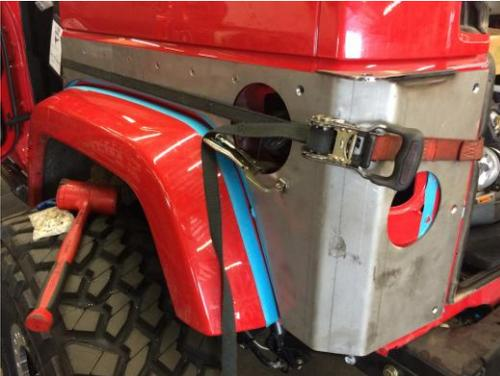
5. Use a large C-clamp through the rear taillight hole in body and clamp RockSkin to body. The use of a good ratchet strap attached to the door striker and tailgate striker will aid in pulling the rockskin to the body. ( See Photo )
