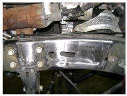
sure tower does not contact steering shaft on driver side.
